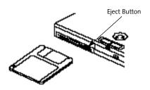
Figure 2-10 Loading/Ejecting a Floppy Disk
